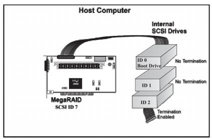
**Terminating External Disk Arrays** In most array enclosures, the end of the SCSI cable has an independent SCSI terminator module that is not part of any SCSI drive. In this way, SCSI termination is not disturbed when any drive is removed, as shown below:
